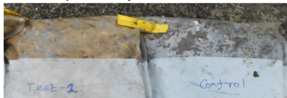
Fig:4 Determination of color and texture changes in 2 kg waste after 30 days of degradation
